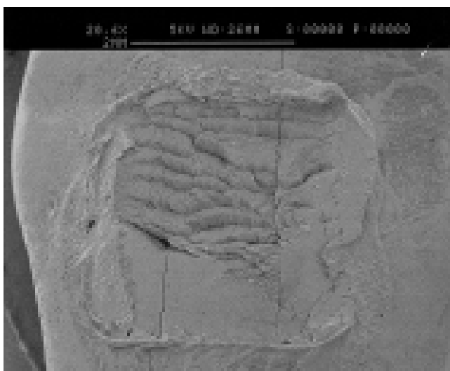
Fig. 3 Scanning electron micrograph of a debonded MCP Bond ® /etched specimen showing fractured enamel surface.
